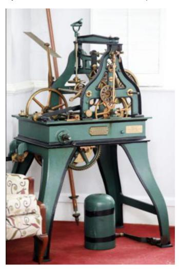
The original clock works at the Church on the Hill in Lenox have been replaced with an automated mechanism and moved to the main sanctuary for visitors to view.
